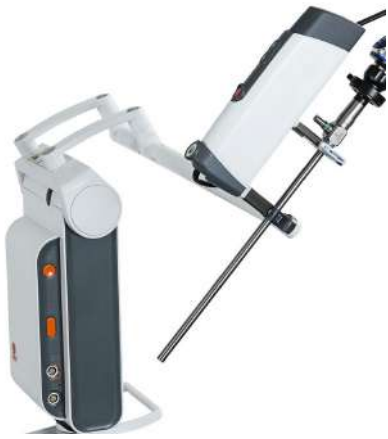
Fig. 3. AutoLap , assistant robot that is capable to control the camera during laparoscopic procedures [17].
